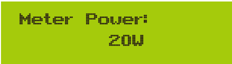
Pic 7.15 Zero-export function via energy meter turn on
