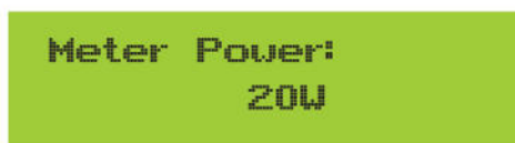
Pic 7.9 Zero-export function via energy meter turn on
